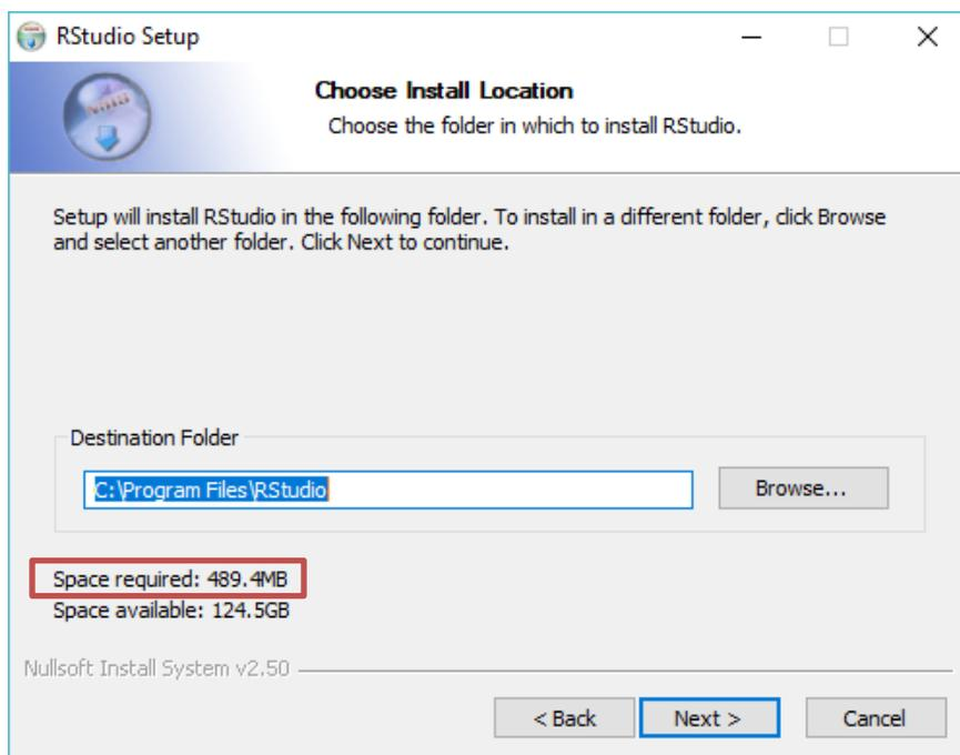
Figure 81. Default *Choose Install Location* window during the RStudio install. Double-check the free disk space requirement and compare against the space available on the computer it is being installed on.
