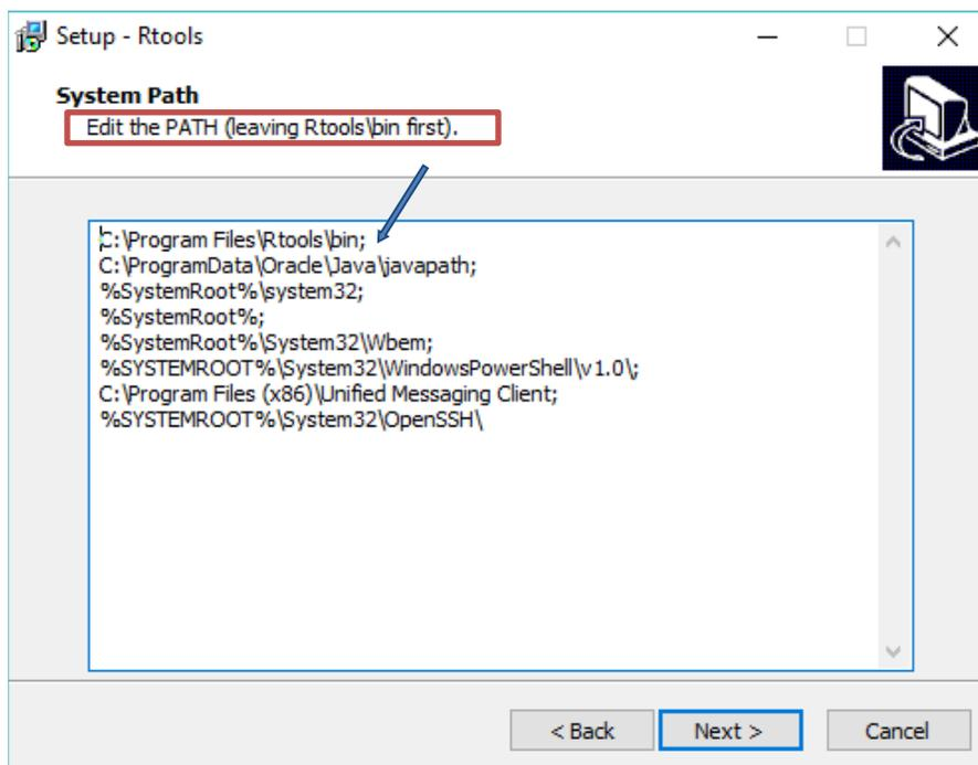
**Figure 73.** The *System Path* window of the Rtools install process. Ensure the path to `Rtools\bin` is correct and the first row of the list.
